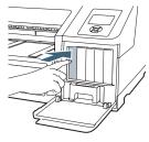
**3** Remove the expended ink cartridge from the printer.
